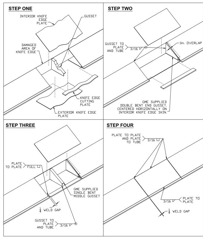
GENERAL KNIFE EDGE REPAIR SPECIFICATION: This specification applies to the following types of trench shields shields:
